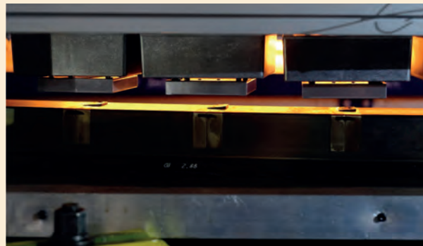
Melting of 3D-reinforcements
