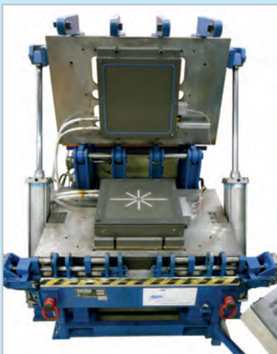
2D-CapaPerm test rig for determining the in-plane permeabilities K 1 and K 2 of reinforcement structures
