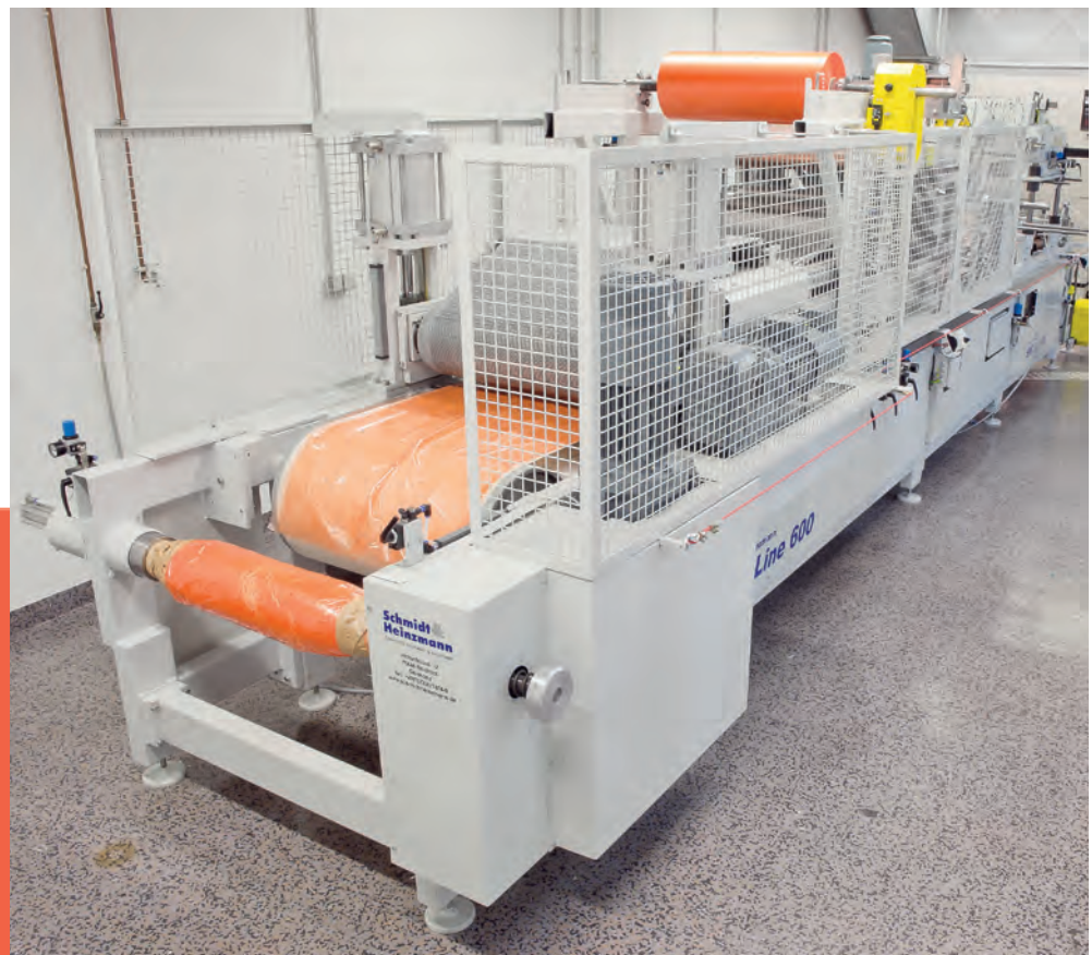
Labor SMC-Anlage SMC facility in laboratory scale
